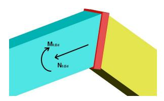
Based on the geometrical characteristics of the nodes, the rule defines a range of connections that can be analytically calculated. The validity range evaluation ensures that the failure modes of the connection will be the same with the expected ones by the rule.
