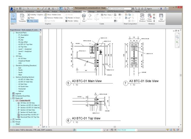
SteelCON is SOFiSTiK Version 2012, 2014 as well as Version 2016 compatible and can be operated within the SSD integrated SOFiSTiK environment. All geometrical and topological data as well as forces can be imported from the overall structure. Connection design results are then a part of the SOFiSTiK Output Report.
