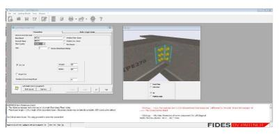
By double clicking a connection in the tree, the user can edit all the geometrical details, and see an interactive 2d or 3d view of the connection, as before. The loadcase editor can be invoked by each input form.
